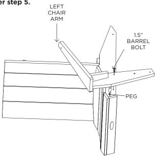
**STEP 3.** Use (2) 1.5" barrel bolts and (2) barrel nuts to attach right & left chair arm to chair back.
